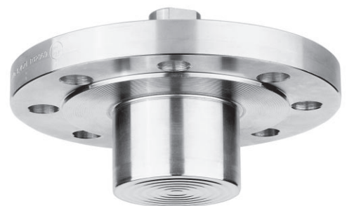
MDM 7515, DN 80, PN 40, Tubus 50 mm
